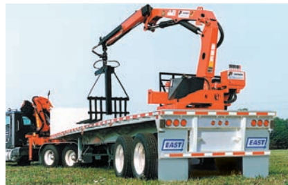
Built-in traveling unloading crane
