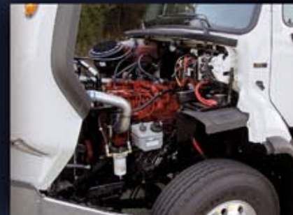
Full tilt hood for easy engine access.
