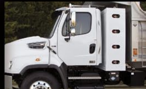
CNG tanks mounted back-of-cab.
