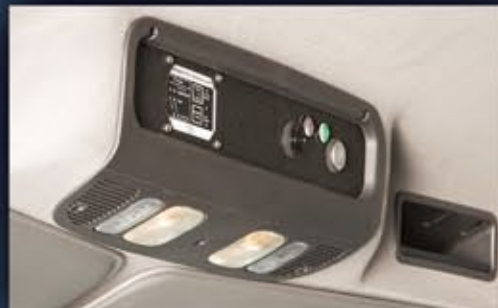
Standard methane gas detection system alerts the driver in the event of a fuel leak.
